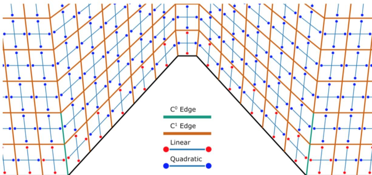
Fig.5: Modified quadratic U-Spline layout. Elements near boundaries (in black) or near  $C^0$  edges (in green) were modified to decrease the degree and increase the characteristic length near the edges. Edges near corners were crease to  $C^0$  to maintain geometric exactness.
