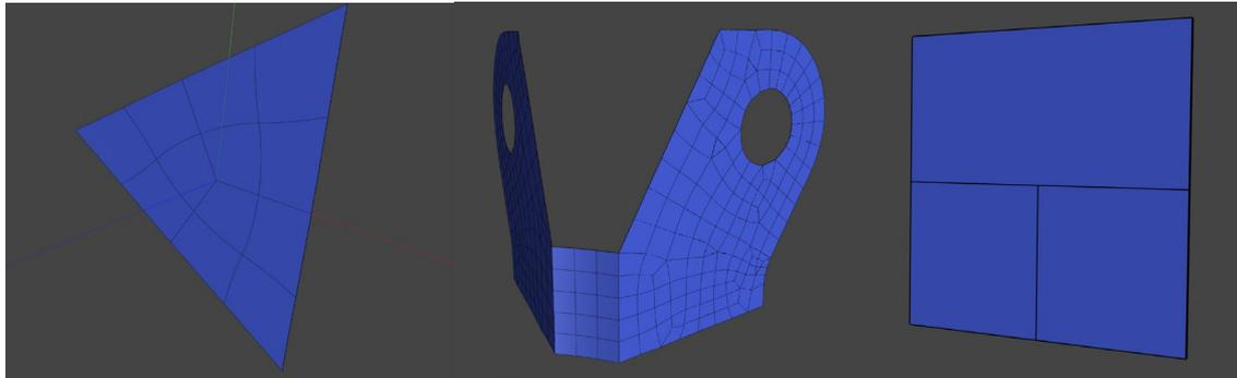
Fig.12: Unstructured meshes read into LS-DYNA. From left to right:  $P=2$  mesh with an extraordinary point,  $P=2$  mixed element types and mixed continuity,  $P=3$   $C2$  mesh with T-junction.
