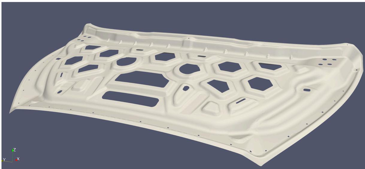
Fig.9: Ford Hood constructed as a  $P=2$ ,  $C^1$  dominant U-Spline
