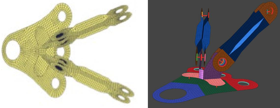
Fig.10: Left: Linear model in LS-DYNA, Right: P2 U-Spline model in Coreform Process
