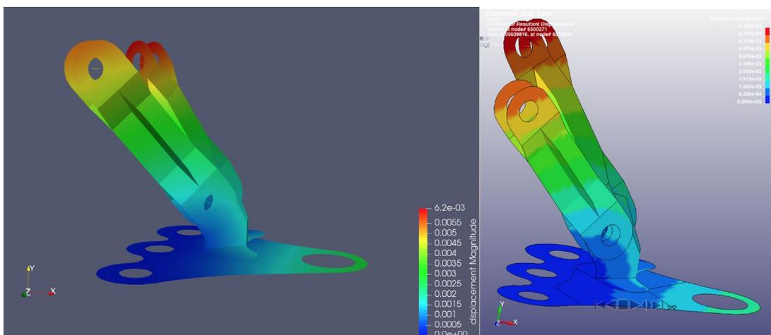
Fig.11: Left: Simulation results of full IGA assembly in Coreform Process, Right: Simulation results of an analogous linear analysis in LS-DYNA
