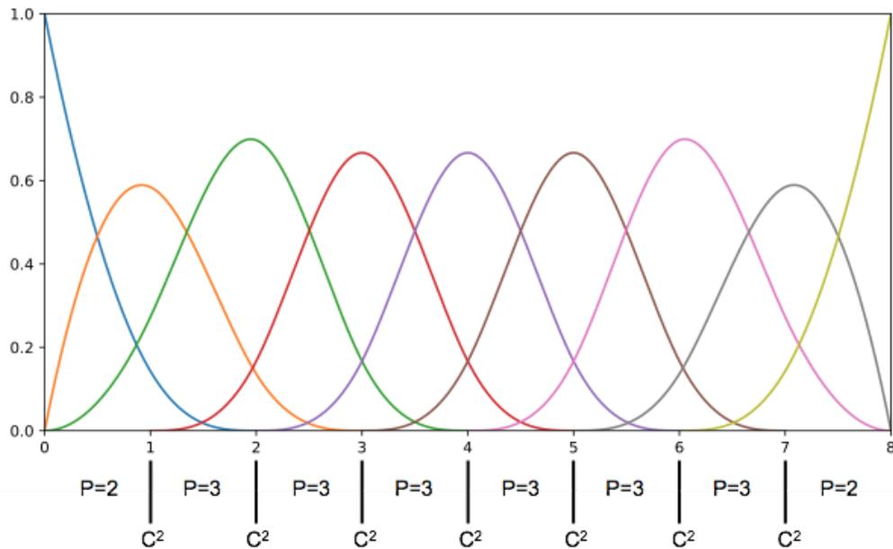
Fig.2: Non-uniform degree U-Spline in one dimension. Novel spline technology permits the construction of bases with varying degree while maintaining properties of partition of unity, linear independence, and positive local support. The U-Spline shown in this figure has been modified at the ends to reduce degree from  $P=3$  to  $P=2$  while maintaining  $C^2$  continuity.
