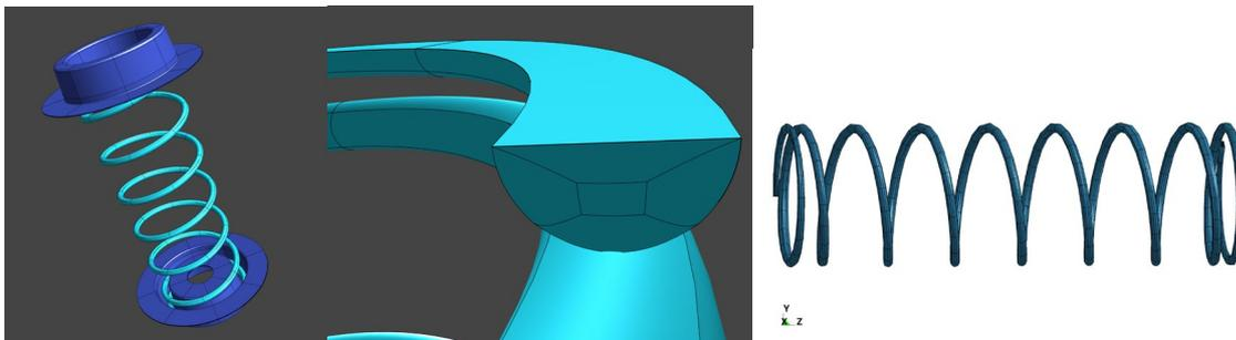
Fig.6: Left to right: Spring contact assembly in Coreform Process, Spring modeled with U-Spline cross section, solid spring geometry in LS-PrePost after export via `*IGA_INCLUDE_BEZIER`.
