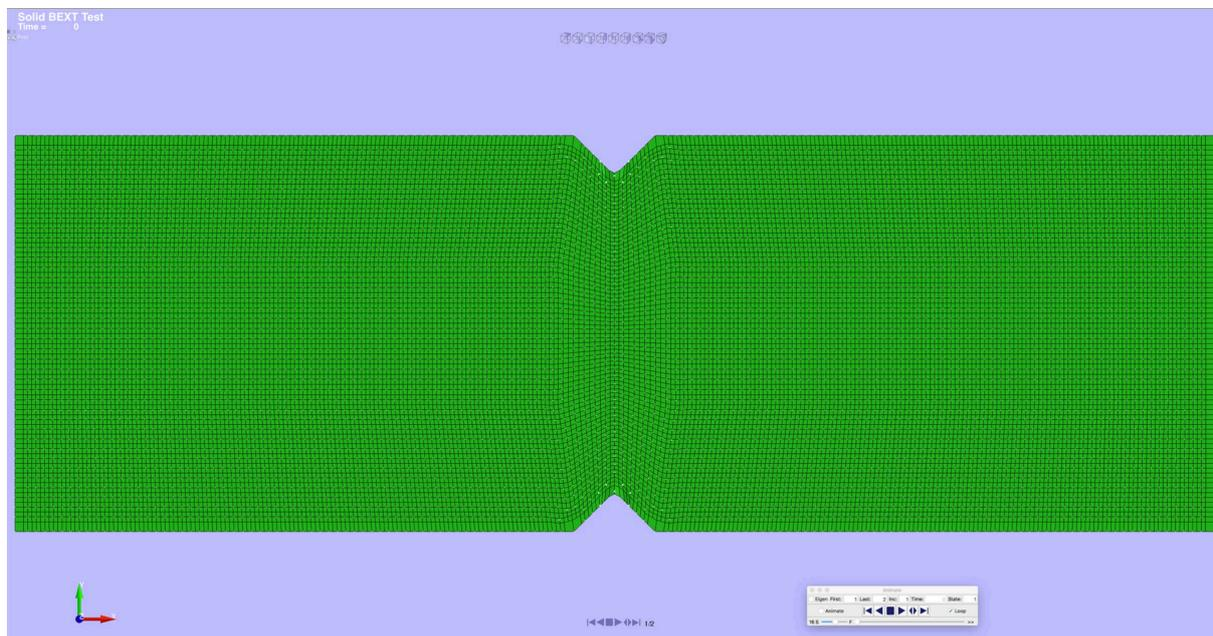
Fig.3: V-notch geometry as a mixed-degree, mixed-continuity U-Spline in LS-PrePost
