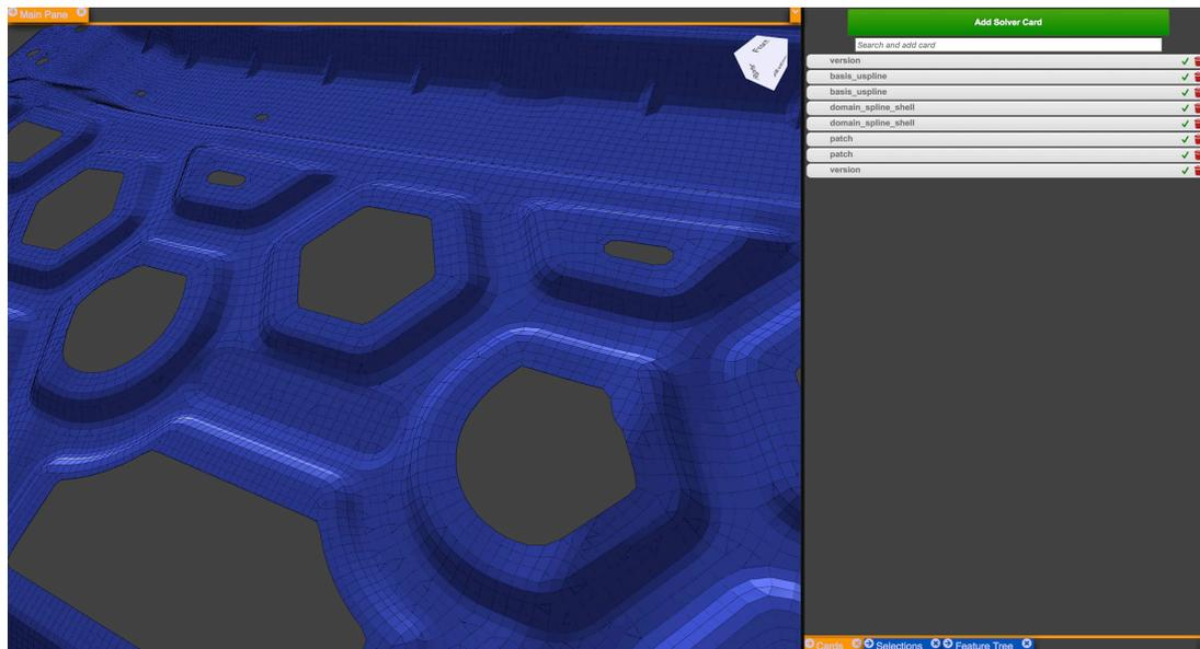
Fig.8: Ford hood geometry as a linear U-Spline in Coreform Process
