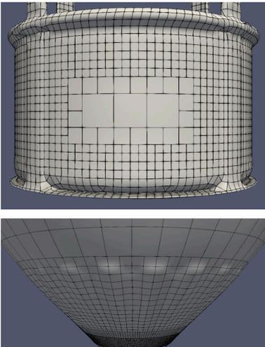
Fig.1: Example of a U-spline model, showcasing the flexible U-spline smoothness and refinement properties critical for success in simulations.
