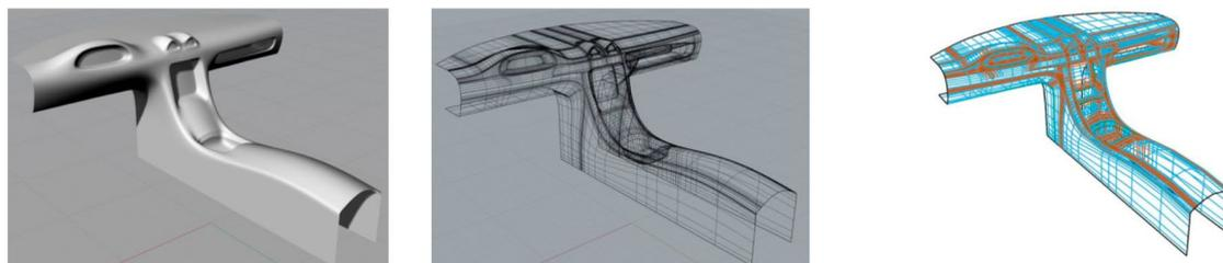
Fig.7: Left to right: Open source automotive console CAD model, model converted to T-Splines, model converted to U-Splines
