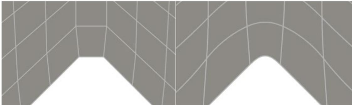
Fig.4: Notch geometry comparison, left: linear finite elements ( $P=1$ ), right: U-splines with modified degree near the boundary ( $P=2$ ).
