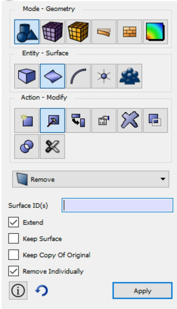
Use CUBIT's **remove surface** command to remove and extend the neighboring surfaces
