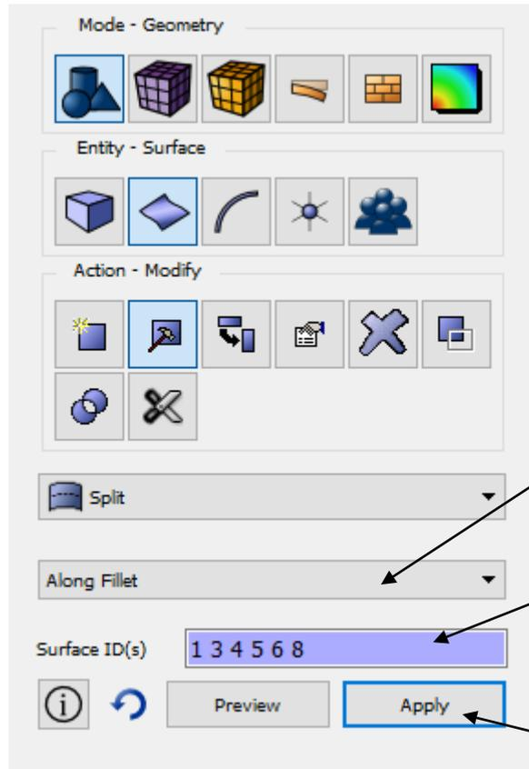
Use CUBIT's **split surface** command to split fillets down the axis of the fillet
