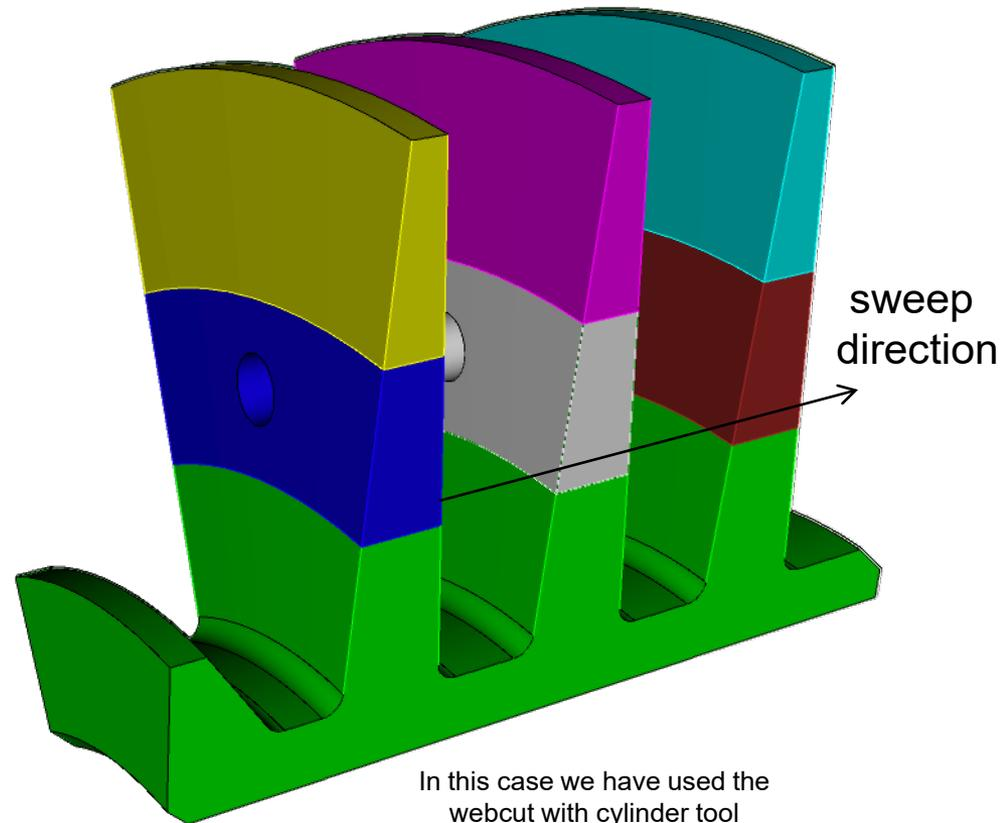
In this case we have used the webcut with cylinder tool
