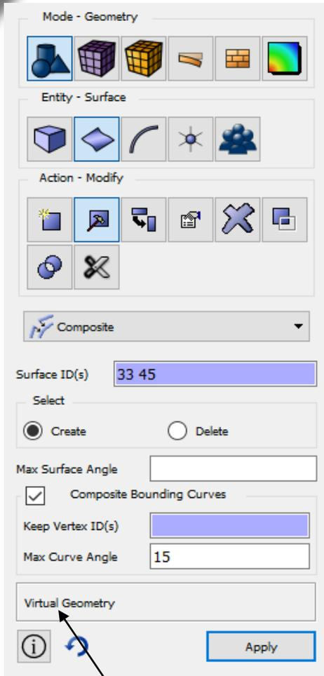
Virtual Geometry is most often used to cover a set of surfaces which normally prevent the volume from being swept.
