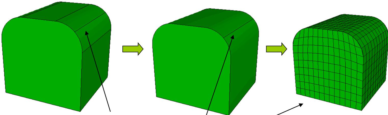
By splitting the surface and then using virtual geometry will result in a higher quality mesh
