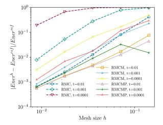
Figure 17: Hyperbolic paraboloid, convergence of the relative strain energy in terms of the mesh size, p = 2.
