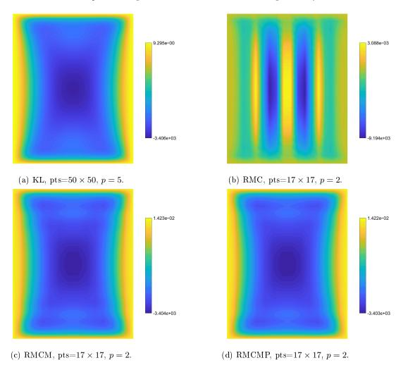
Figure 13: Scordelis-Lo roof, membrane force  $n_{\phi\phi}$ , t = 0.25, maximally smooth elements.
