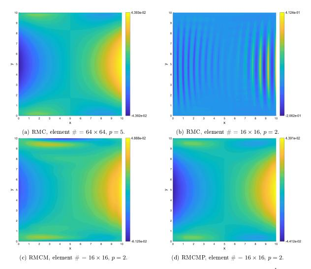
Figure 10: A clamped square plate under distributed load, shear stress  $\sigma_{xz}$  at the midsurface,  $\frac{L}{t} = 100$ .
