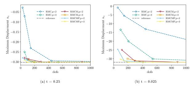
Figure 12: Scordelis-Lo roof, convergence of the maximum displacement, p = 2, 3, maximally smooth elements.
